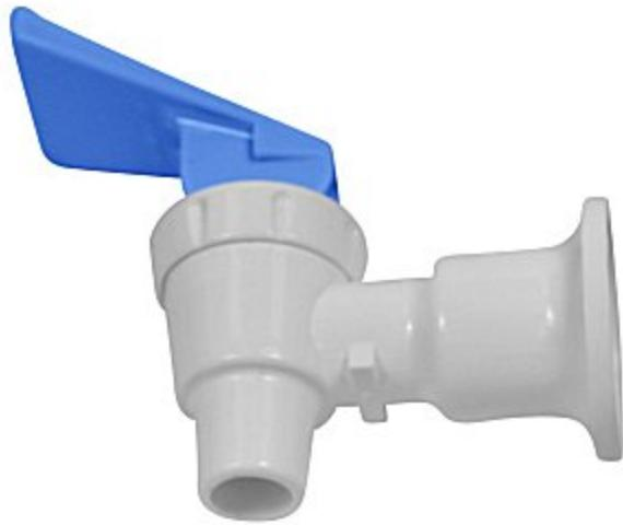
White Body with Blue Handle Sunbeam Replacement Water Cooler Tomlinson Faucet Handle, white polypropylene body with internal 3/8"-18 NPS threads and 05" (1 mm) recess for washer in the back of the flange.
