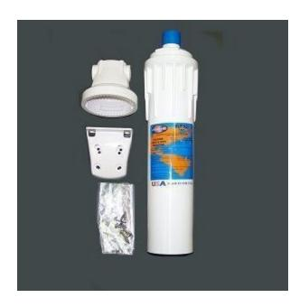
Taste, Odor, Scale, Sediment Filter. Bracket, Head, And Screws. 10 inch Cartridge 1.65 Gpm, 13,000 Gallons life, 3/8 Fpt Head., Replacement For Wilbur Curtis, CSC10AC00, 1360101329
