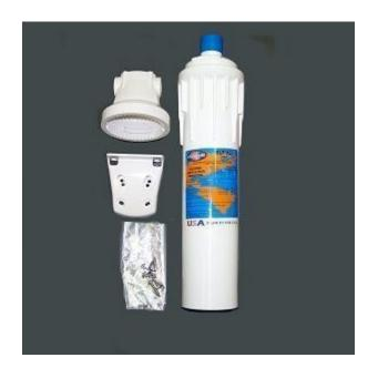
Taste, Odor, Scale, Sediment Filter. Bracket, Head, And Screws. 10 inch Cartridge 1.65 Gpm, 13,000 Gallons life, 3/8 Fpt Head., Replacement For Wilbur Curtis, CSC10AC00, 1360101329
