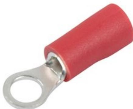
This series is the most economical insulated terminal available. The PVC insulation sleeve is securely fastened to the butted seam barrel. The insulation has a flared entry for easier wire insertion. Rated 600 volts maximum, building wire; 1000 volts maximum, signs and fixtures. Industry standard color-coding indicates wire range. Temperature rating: 105° C (22
