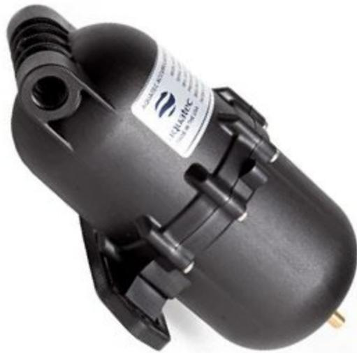
Convenient 3/8" Female NPT ports. Compact design fits in small spaces, Dimension 8.92" L X 4.84" W X 4.13" H Dampens pump switch cycling/pulsations. Limits harmful spikes/water hammer. Minimizes hydraulic noise NSF food grade materials Easy to install and maintain Mounts in any position with included bracket. Maximum Working Pressure - 125 PSI. Pre-Charge - 20 PSI
