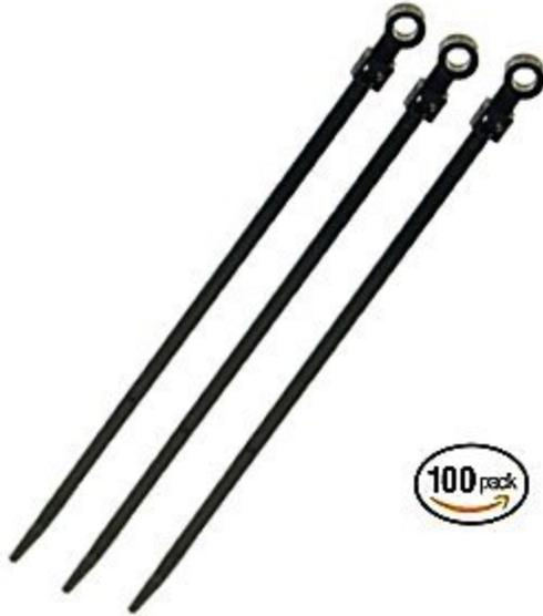
Mounting tab cable ties have a molded-in screw hole for securing bundles of wire on virtually any surface that has or can accept a drilled hole. Up to a 1/4-in screw size can be used, or a comparable rivet size. All mounting tab cable ties are made of durable 6/6 nylon. For use at temperatures not exceeding 85° C (185° F). Recognized under UL file #E125869(N). Meets UL94V-2 Flammability Classification.
