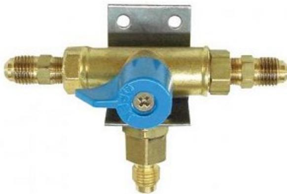
Economy Low Pressure Changeover Valve Switch cylinders without service interruption. Low cost alternative to high pressure and auto changeovers. Has 1/4" male flare back check inlets and 1/4" male flare outlet. Requires 2 C02 regulators.
