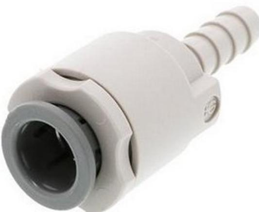
John Guest Superseal Incorporates Hand Operated Nut To Apply Extra Pressure To Tubing, Also Double O-Ring System. Gray Acetal Copolymer Construction, Nitrile O-rings, FDA Approved Materials, NSF Certified 51 & 61, Designed For Use With Stainless Steel Or Copper Tubes, Suitable For Potable Liquids And Food Applications. Bags Of 10 Or Each, Max Temp 150°F, Max Pressure 150 Psi At 68°F.
