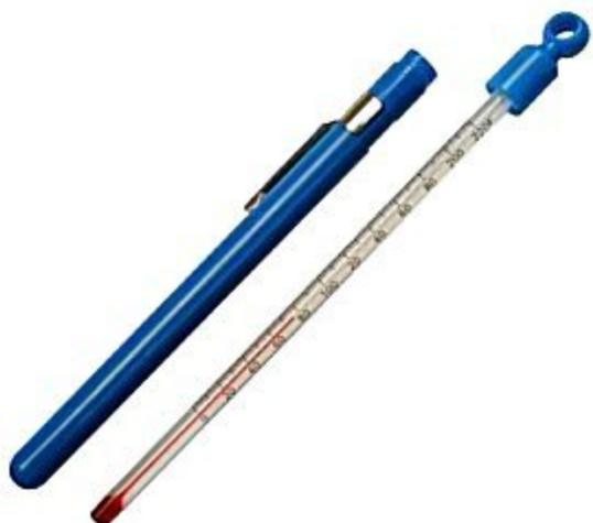
Non Stock Must Be Ordered. Non Toxic Liquid In Glass Thermometer, Temp. Range 0-220°F , Length 6.25 In., Immersion Depth 13mm, Scale Divisions 2 Degrees , Includes Pocket Clip,
