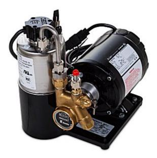
McCann Small Carbonator, Water Capacity, 100 Gph Maximum, Tank Capacity, 32 Oz Stainless Steel, Electrical, 115V/60hz/1phase, Soda Outlets 1, ASSE 1022 Compliant
