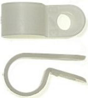
Nylon cable clamps are tough, resilient, lightweight, and resistant to aging and most chemicals. Mounting hole is 13/64 inch diameter. Recognized under UL File. Meets UL94V-2 Flammability Classification.
