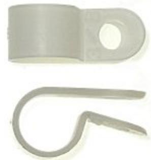
Nylon cable clamps are tough, resilient, lightweight, and resistant to aging and most chemicals. Mounting hole is 13/64 inch diameter. Recognized under UL File. Meets UL94V-2 Flammability Classification.
