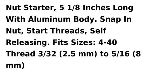
Comes With Pocket Clip. Use on all small size nuts to start nuts on bolt thread. Releases from nut as threads are engaged.
