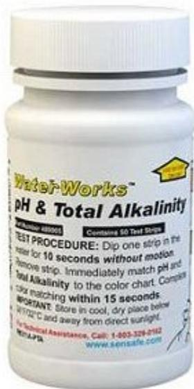
pH & Total Alkalinity test is a single test strip that has been designed with two separate test pads: one for pH and the other for Total Alkalinity measurements. This test is an alternative to wet chemical tests since it gives reproducible results for each test separately. Test range is from 6.0 to 9.0 for pH and 0-360 ppm (mg/L) for total alkalinity. pH: 6.0, 6.5, 7.0, 7.5, 8.0, 8.5, 9.0, TA: 0, 80, 120, 180, 240, 360 ppm
